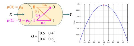
Figure 10: Maximization of mutual information to find capacity of a BSC channel. Capacity of 0.029 bits is achieved by  $\mathbf{p} = [0.5,\ 0.5]$
