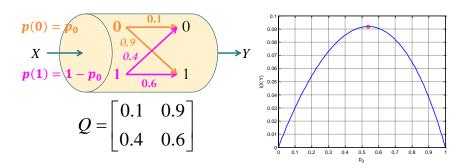
Figure 9: Maximization of mutual information to find capacity of a BAC channel. Capacity of 0.0918 bits is achieved by  $\mathbf{p} = [0.5376, \ 0.4624]$
